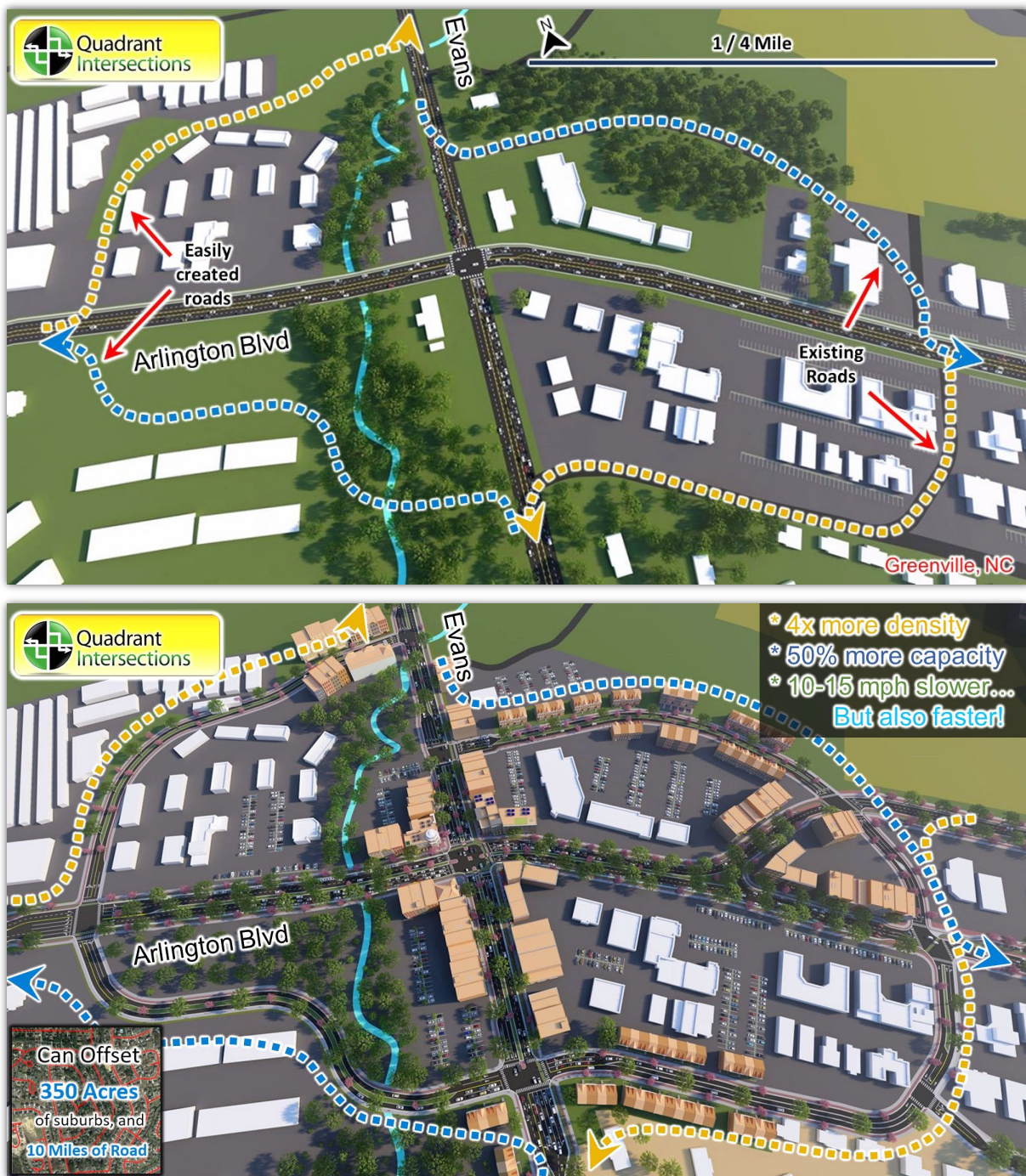
Figure 4-6 Four Quadrant concept for Arlington Blvd and Evans Street in Greenville
