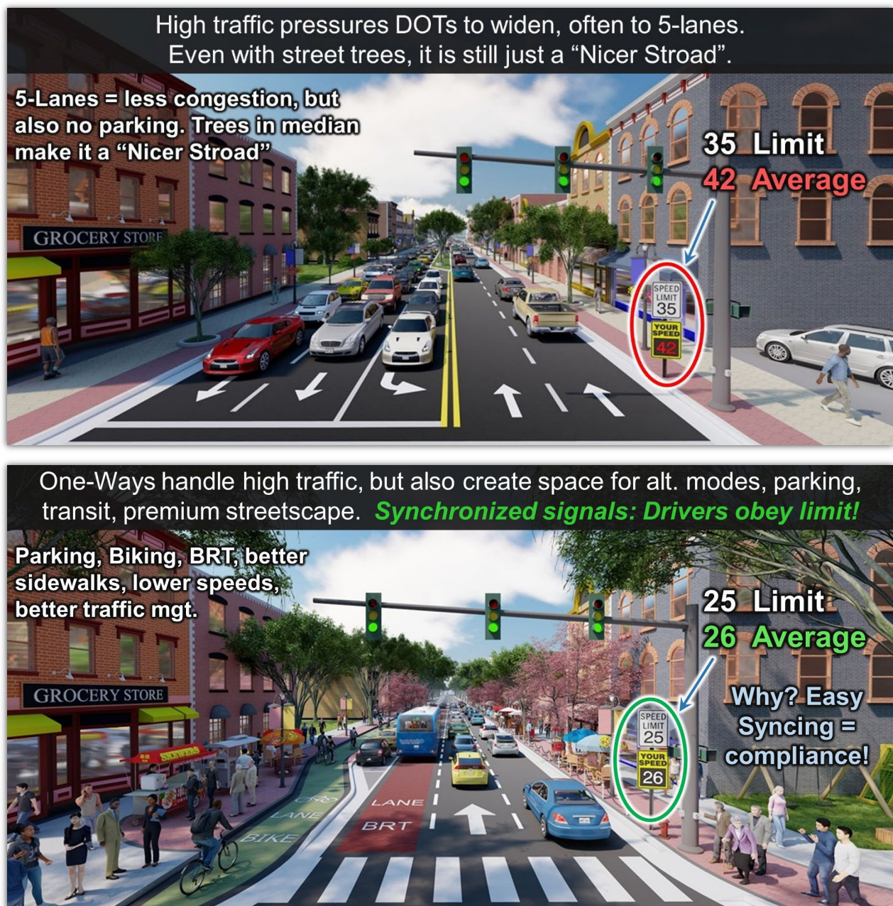
Figure 5-5 Drivers likely obey speed limits, even if slow, due to perfect synchronization.
