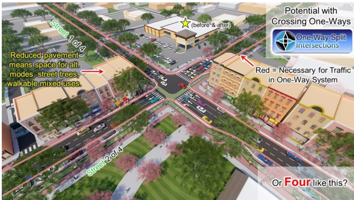
Figure 5-12 Same Location, Reconfigured with four One-Way Streets
