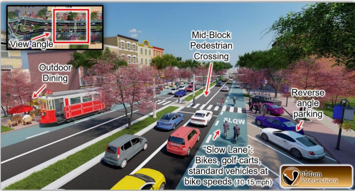
Figure 4-3 Closeup view of the “Slow Lanes” concept
