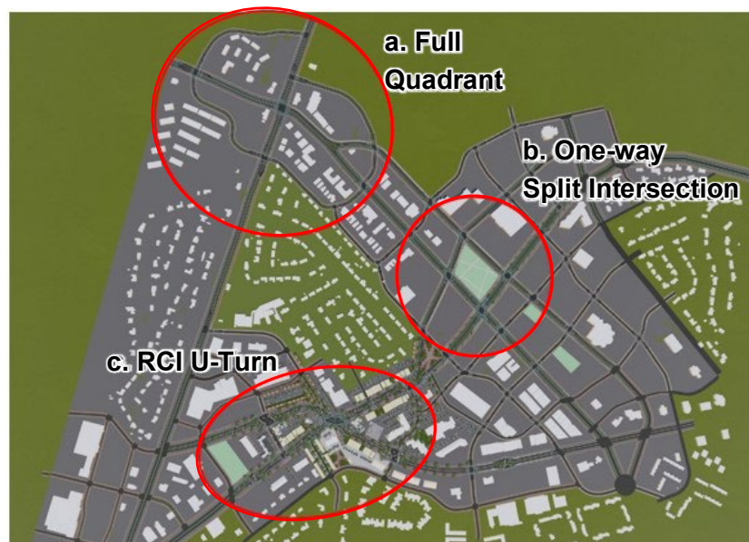
Figure 6-3 Proposed Alternative Intersection Designs
