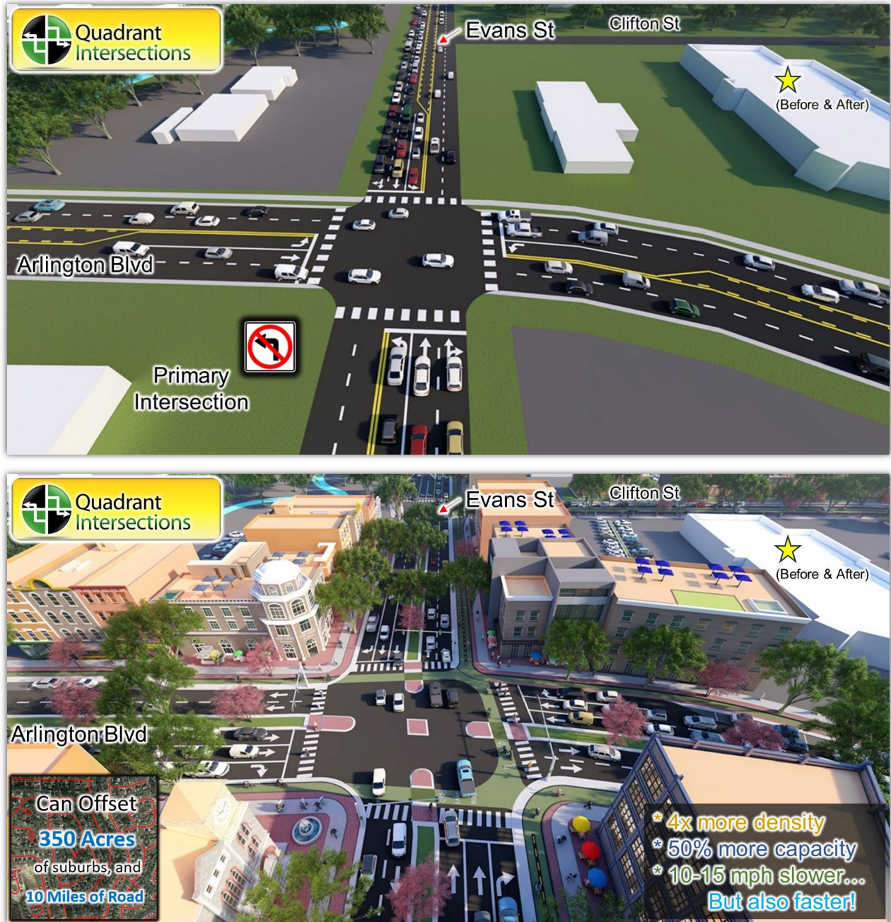
Figure 4-8 Four quadrant concept at Evans Street & Arlington Blvd: Closeup of primary intersection.
